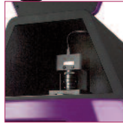
High resolution 5MP scientific camera captures high resolution images and allows analysis between closely located bands or spots
