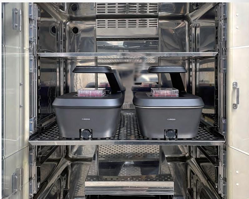
**Celloger Mini Plus** is equipped with advanced fluorescence and bright-field technology providing the highest quality images and time-lapse videos. Various cell-based research workflows and applications such as wound healing assay, cell proliferation, cytotoxicity assay, transfection efficiency, co-cultures, cell growth and confluence can be examined using this all-around system.
